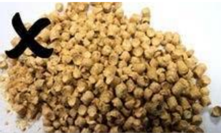
Pellets too short in length
